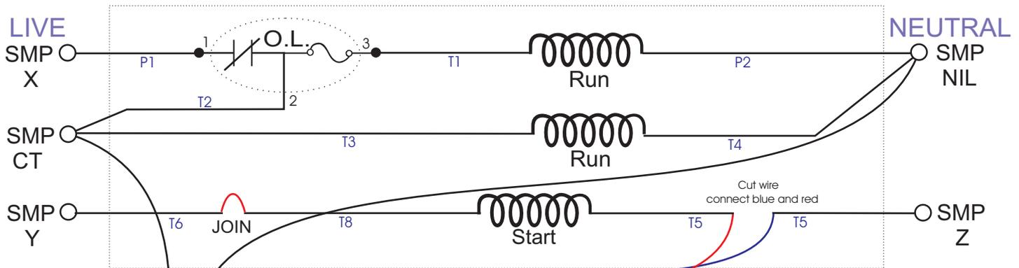
Note: wires T5 and T8 can be reversed
