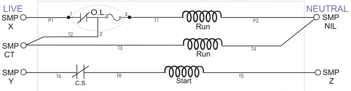
The RED and BLUE wires of the Solid State Start Switch take the place of the mechanical start switch.
